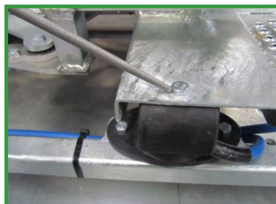
12. Secure Loadbar to Cradle with 2 x M10 x 25 Bolt
