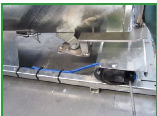
11. Secure Loadbar Base with 4 x M10 x 30 Bolt and Nut
