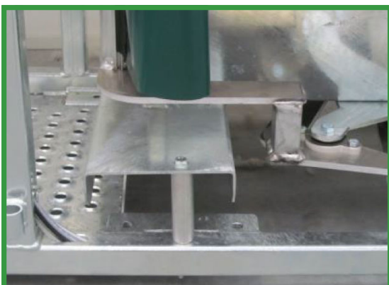
9. Remove packers (90mm tube) at the exit end of the Autodrafter
