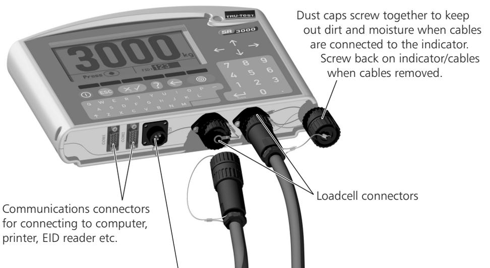
Communications connectors for connecting to computer, printer, EID reader etc.
